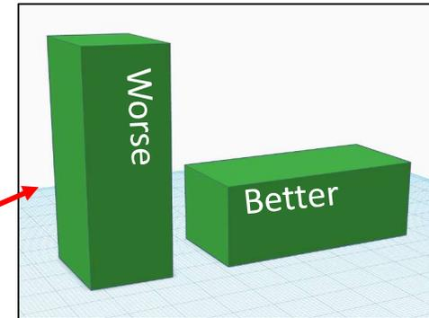
Try to rotate the part so the smallest dimension is vertical. It's stronger that way, and it builds faster.
