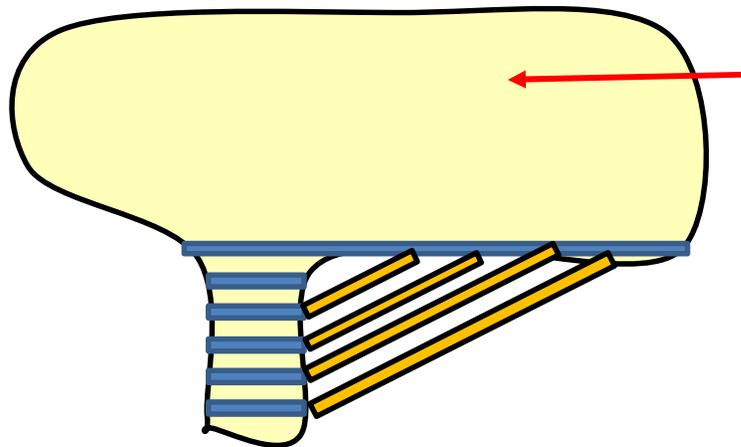
Some 3D printers handle this by using software to add “support structures” to the overhangs
