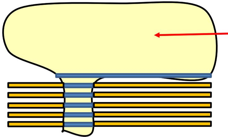
Some 3D printers handle this by leaving unused material in place to support the overhangs
